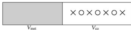
Fig. 15.27 Complete phase-separation into two large clusters (metallic and charge-ordered). V_m and V_{\text{CO}} are the volumes of the two clusters [8]
